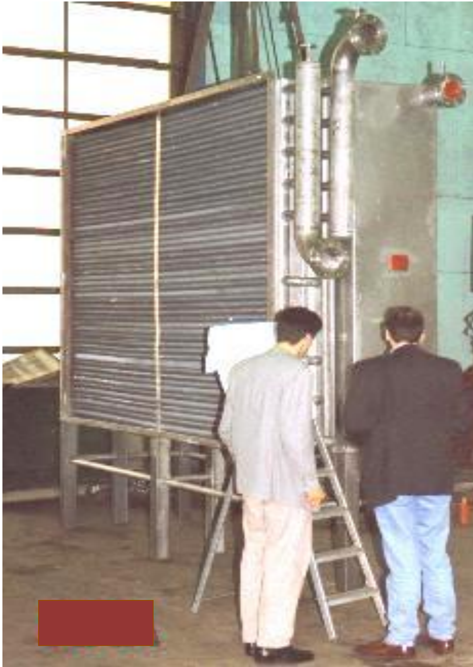
Oil to Hot air radiator using HTO - Process air heat exchanger
